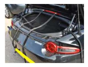
2. Place the anti-slip matting towards the front of the boot/trunk-lid (i.e. Near to driver. Ensure the boot/trunk lid is clean)
