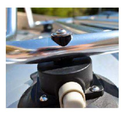
Do not fully tighten the bolt ensure the vacuum cup can rotate freely on the frame before you fit the rack to your car. This allows the cups to rotate on the frame to fit the curve of your cars boot/ deck lid.
