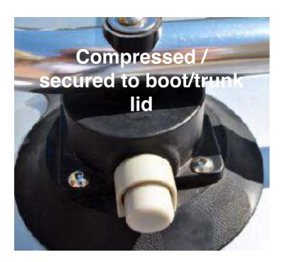
5. You must ensure that all the vacuum cups have a secure fit and that they stay compressed. We recommend after 5-10 miles with the rack loaded you stop and check the vacuum cups. Its easy to see if they have leaked and are not compressed as the red line will re appear on the plunger. The vacuum cups are not intended to be permanent fixtures on your car they will lose vacuum slowly over time.
