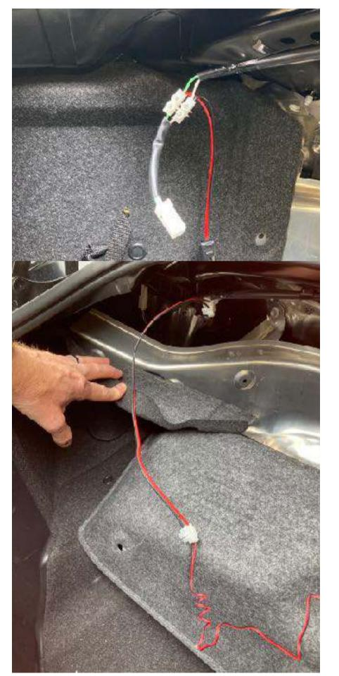
Disconnect the plug. You can see the cable running at the back of the boot up the light at the rear of the boot lid.
