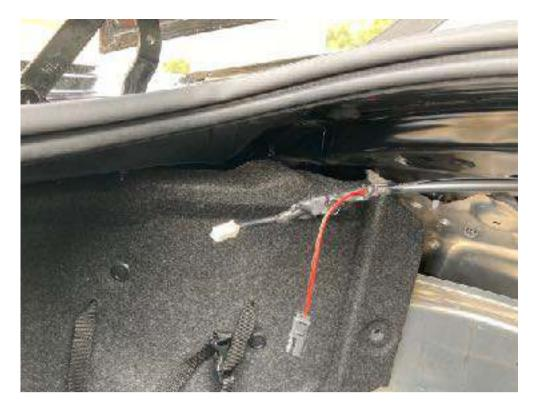
Connect the spur via the terminal block then wrap the joint in insulation tape.
