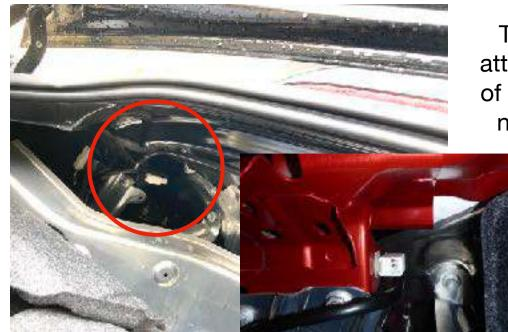
The third brake light on a MX5 ND attaches to a plug at the top back left of the boot. The carpet on the left will need to be pulled away to reveal it
