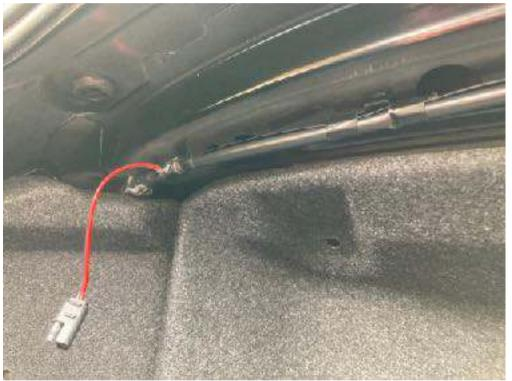
Reconnect the wiring to the socket on the left and you are left with a connector that at any time you connect the third brake light too.
