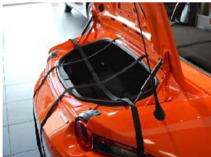
Lay the straps out as shown the long strap left to right
