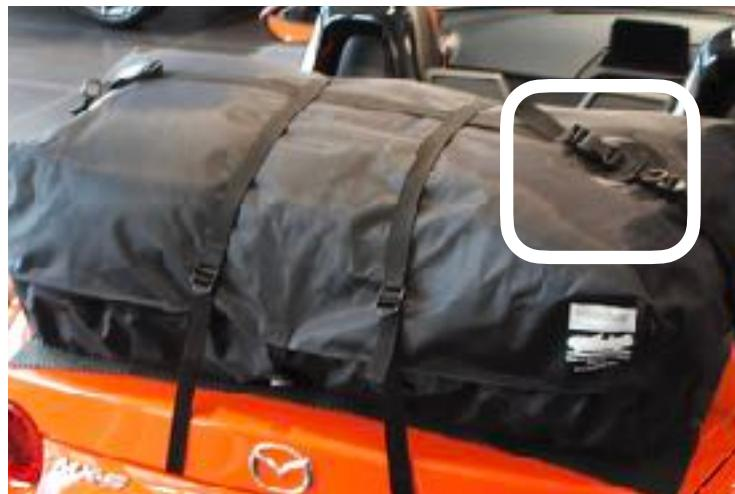
Fit the H shaped strap, click this into the fixings on the top of the bag left & right.
