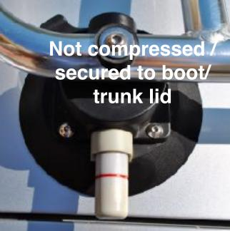
4. Once all the vacuum cups are fully compressed, the red line will disappear as below. Now fully tighten the bolts ensuring the rack is tight on to them (leaving them loose to start allows them to curve to your trunk/lid and ensure a good compression of the cups)
