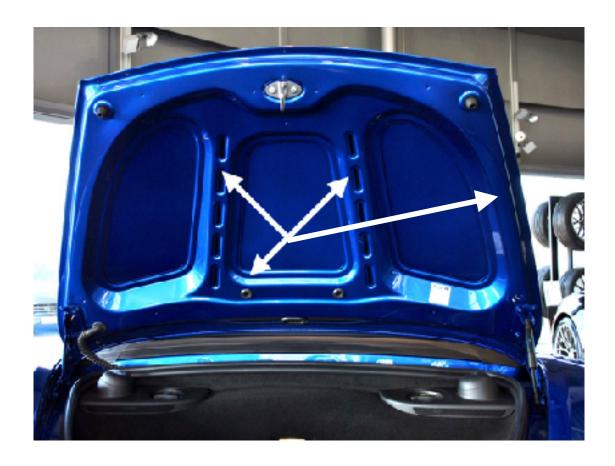
3. Make sure you wipe the cup base and area the cup will attach to on the trunk/boot lid with a damp cloth prior to fitting. This protects paint and stops air leaking. Press down on the rack above each cup and pump the air out of the vacuum cups using the plunger. The red line will disappear when the cup is fully compressed. You may need to press firmly to secure the cup, make sure the cup is loose on the frame so it can rotate.
